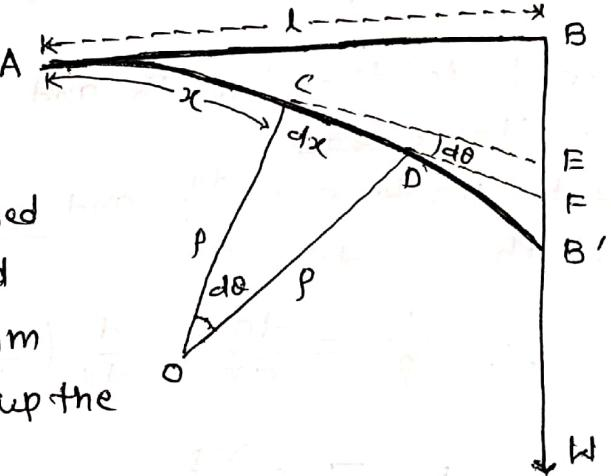
Consider a section of the beam at C distance  $x$  from the fixed end A of the cantilever.
